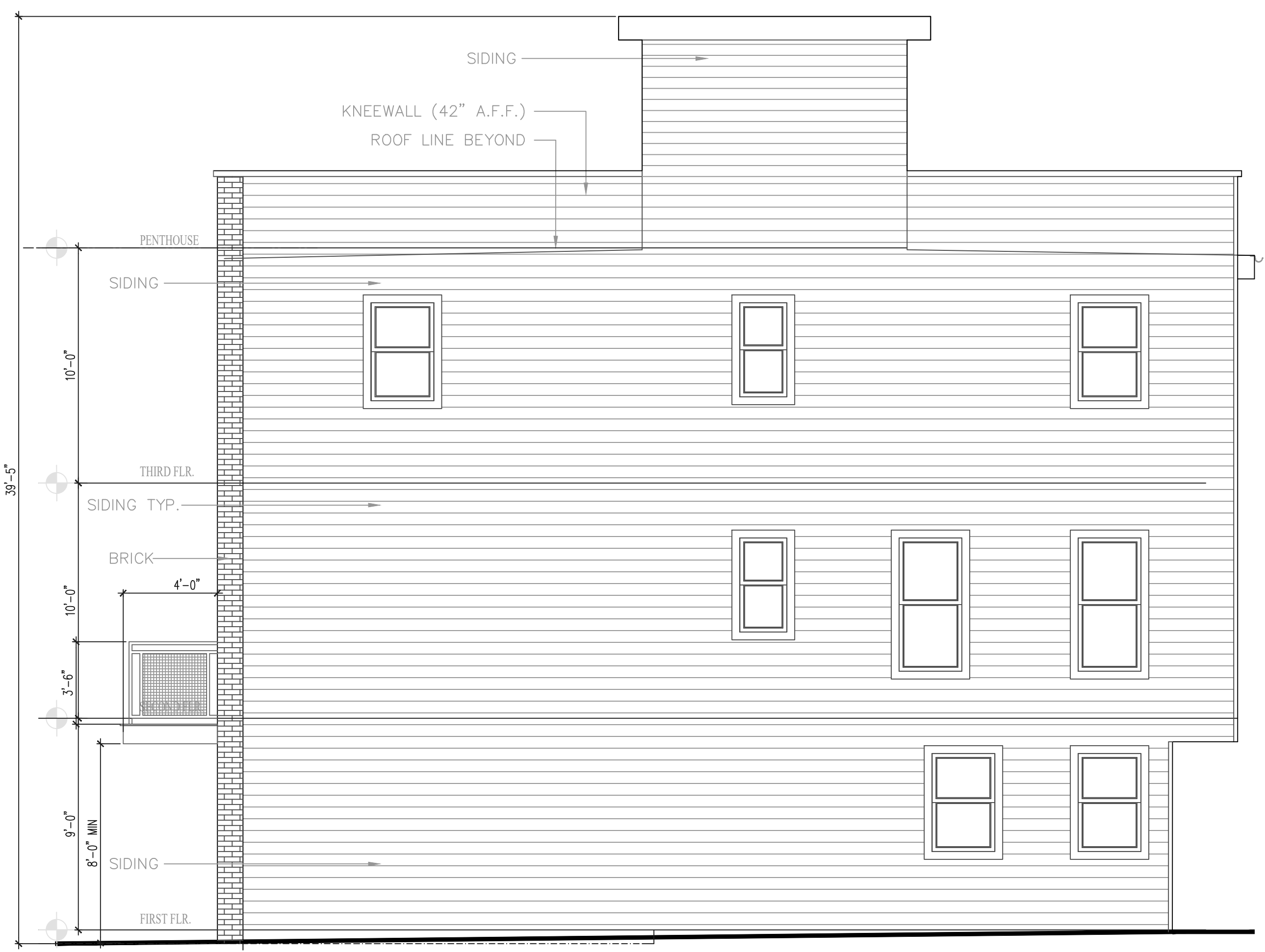
SIDE ELEVATION (ROPEWALK LANE)
